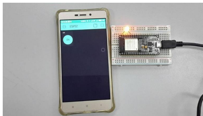
Figure 11: Blynk app with ESP 32
