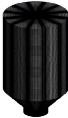
Fig.3 Compute domain grid for water flow experiment equipment
