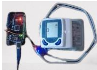
Fig. 3. Data acquisition from Blood pressure and Heart rate sensor.
