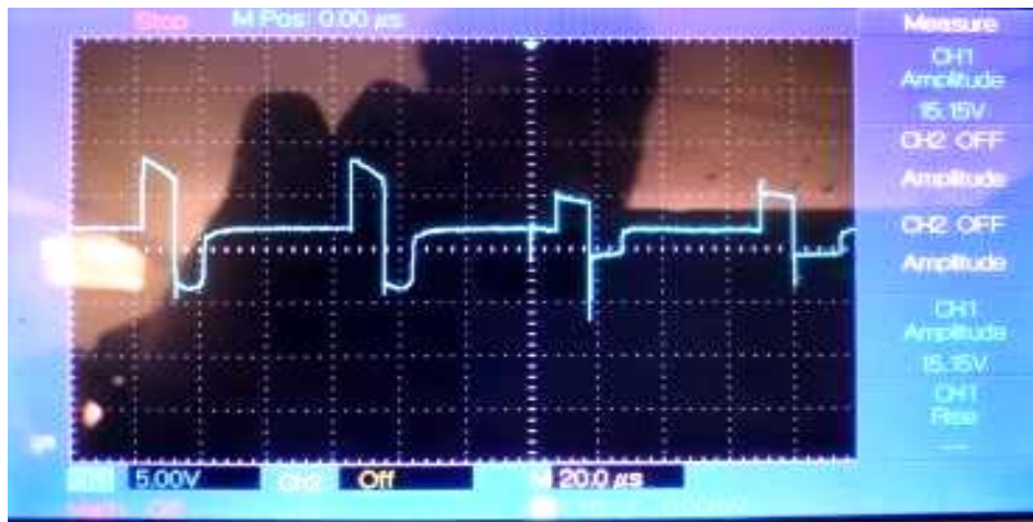
Figure 4.3: Voltage waveform at voltage level 5V
