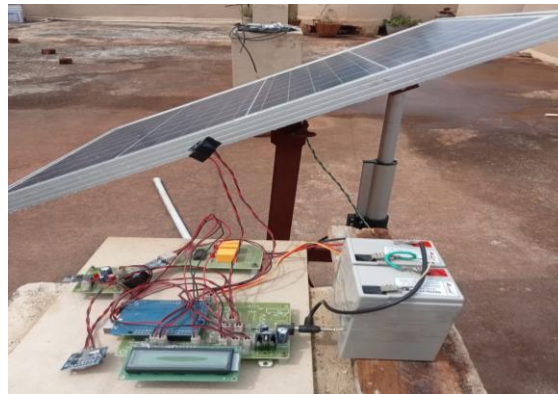
Figure 14: Actuator used for tilting the solar panel and Relays used to operate the solar panel tilt in both directions using clockwise and anticlockwise shifting
