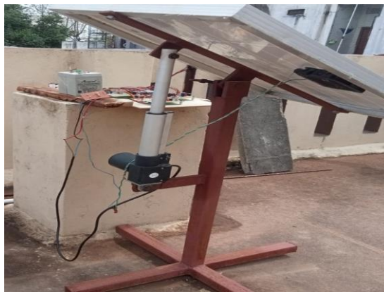
Figure 13: Mechanical setup for tilting the solar panel
