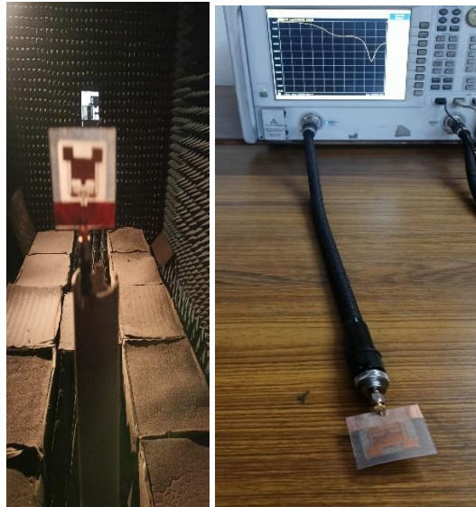
Fig. 8 Measurement setup of Antenna
