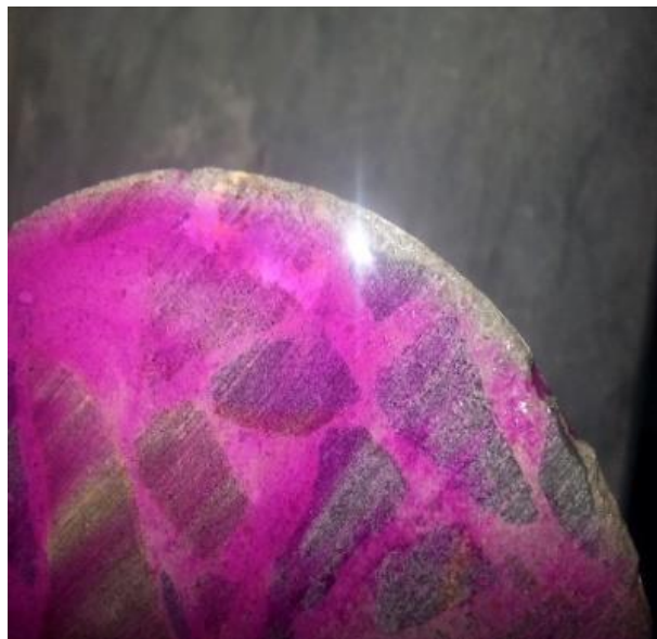
Figure 5. Phenolphthalein carbonation test result.
