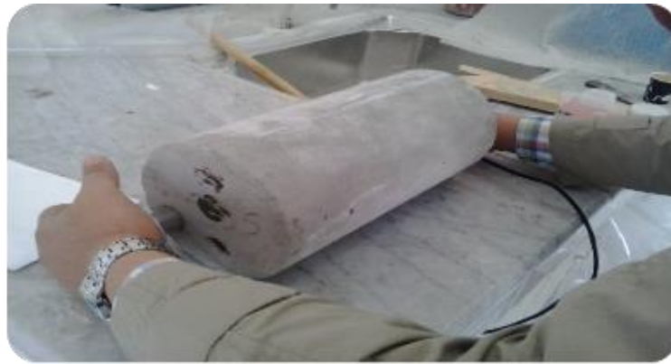
Figure 4. Non-destructive measurements, Ultrasonic testing.
