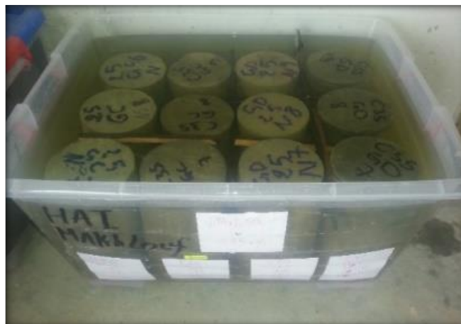
Figure 2. Storage of test specimens in an aggressive environment.
