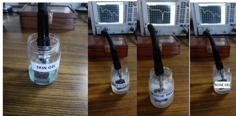
Fig. 8. Experimental setup for mimicking gel for skin, fat, muscle, and bone phantom.
