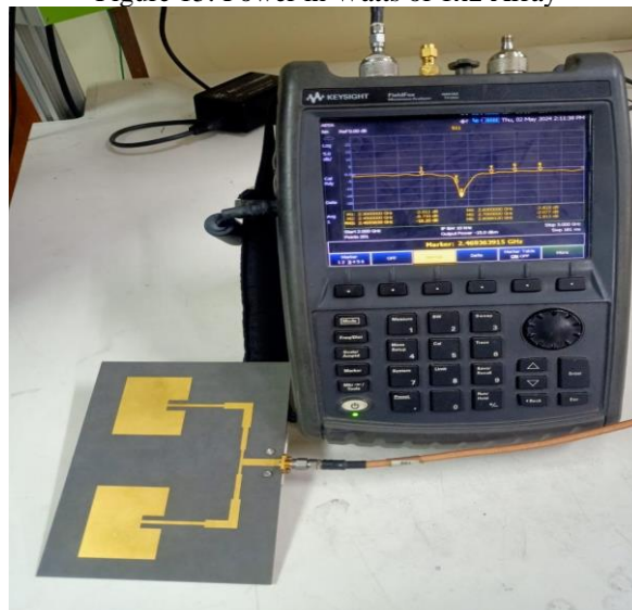
Figure 16: Measuring Return Loss of 1x2 Patch Array Antenna
