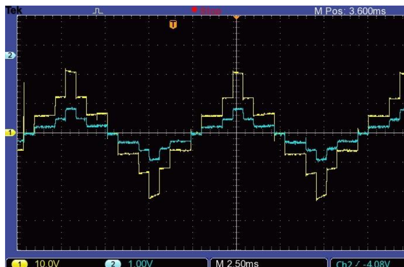
Fig. 12. R load (100 Ohms) hardware waveform of renewable energy based MLI
