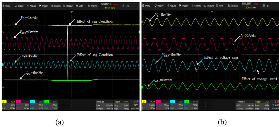
Figure 9. (a-b) Condition of dynamic voltage sag: P CC1 voltage, load voltage regulation, series VSC injected voltage, dc-link voltage, P CC1 current, and PV array current.
