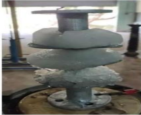
Fig 1. Icing On Insulator
