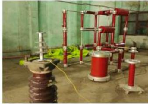
Fig 4. Experimental setup for lightning and switching impulse withstand tests
