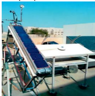
Figure 8 PV with a pyranometer
