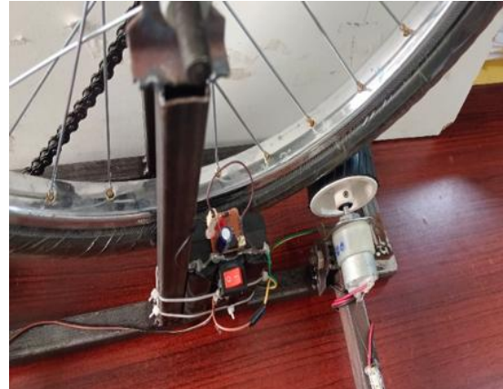
Fig3. A Close View of Circuit Connections of Regenerative Braking in EV.
