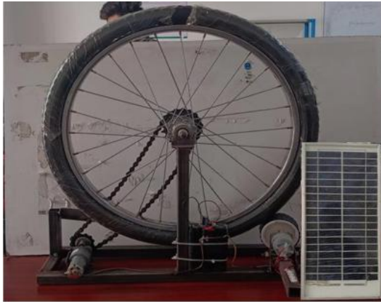
Fig2. Experimental Setup of Regenerative Braking in EV.
