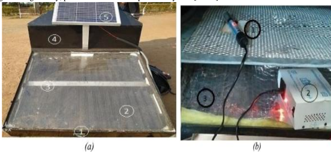
Figure 15. A hybrid solar dryer uses light sources during the day and dark during the night. 1) Compressor; 2) Plates of glass; 3) Confusion, 4) The drying box 5) Solar panels 6) Coil for heating 7) The inverter 8) Foam
