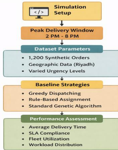
Fig 3: Simulation and evaluation procedure for the proposed optimization model, detailing the experimental setup, dataset parameters, baseline strategies, and performance assessment criteria.
