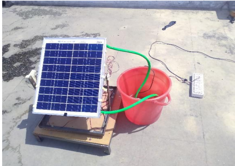
Fig.2: Measurement of voltage and current of solar thermal photovoltaic
