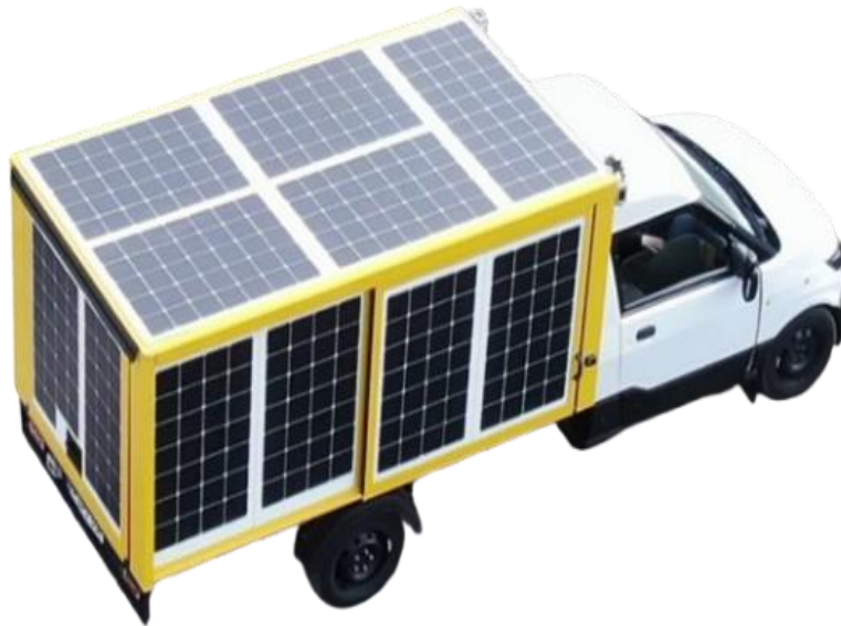
Figure 1: Electric Vehicle integrated with PV array
